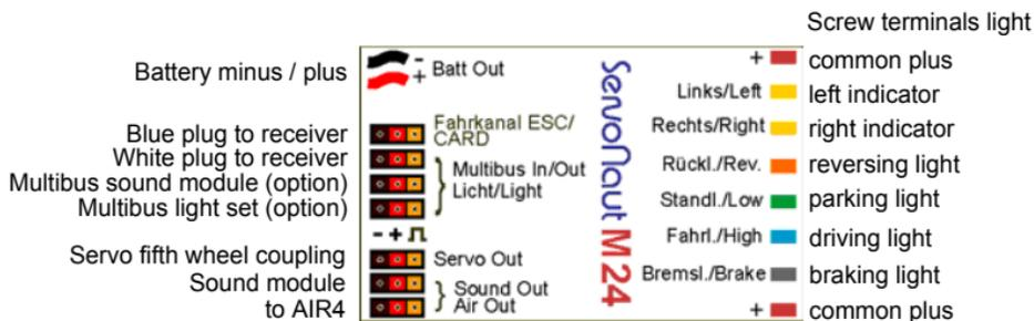
The M24 type plate is also used as a heat sink. The module might heat up and need some cooling. Don't cover it with foam!
