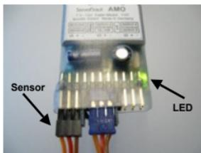
*Installation of the IR transmitter (in the tractor) and IR sensor (in the trailer) is not difficult, they don't have to be perfectly aligned. But keep the distance under 15 cm. Because of the wide transmission angle of the transmitter and the high sensitivity of the sensor the link will work also in tight curves.*
